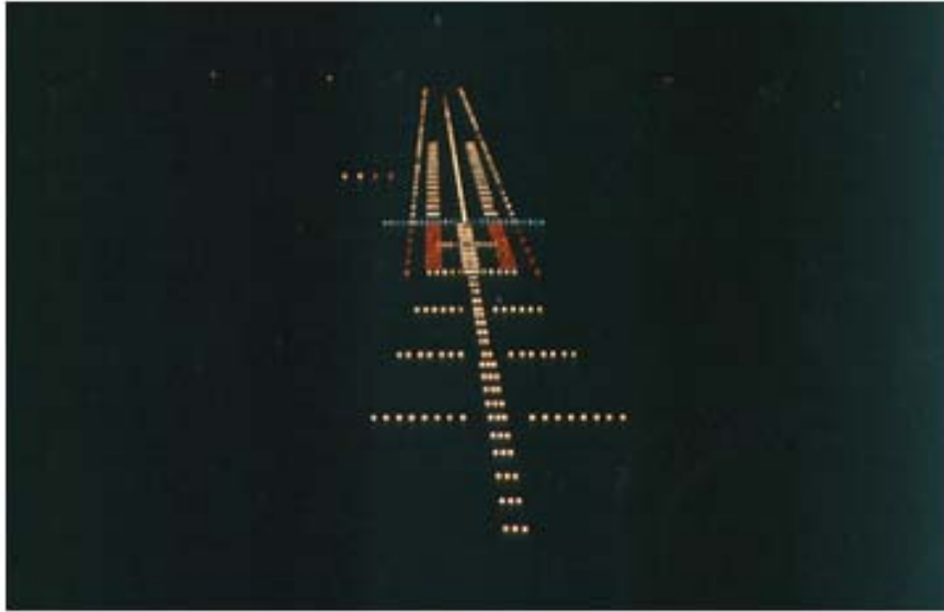
Figure 1. Aeronautical ground lights (approach & runway lights) as seen by the pilot on approach to land at a major aerodrome
